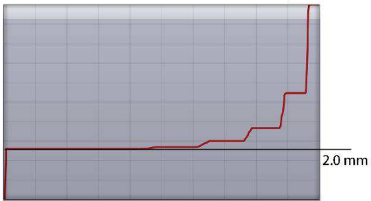
Fig. 5 Visualisation of the deviation from layer height for both trajectories using a plot of distances between all adjacent points and coloured visualisation on the mesh
