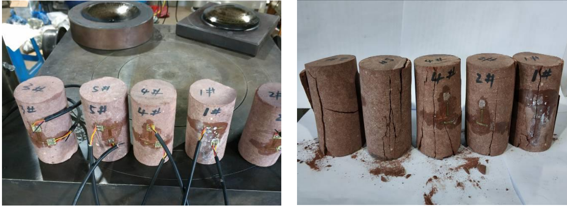
Fig 5 Standard rock sample and broken state after test
