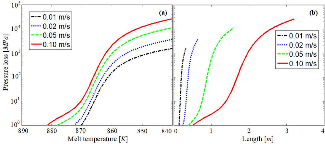
Fig. 7 Variation of pressure loss (a) with the decreasing melt temperature and (b) along the filling length at different filling speeds.
