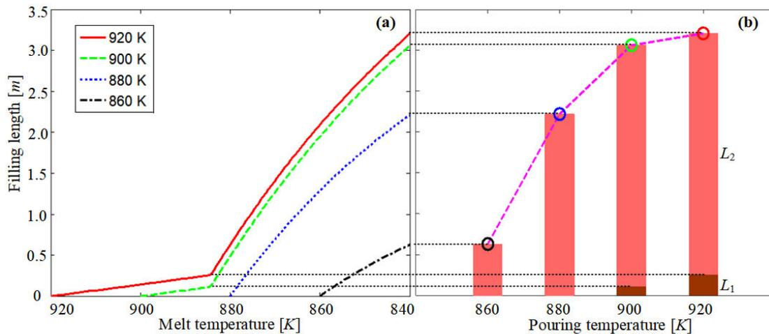
Fig.5 Relationship between the melt temperature along the spiral channel and the filling length at different pouring temperatures.
