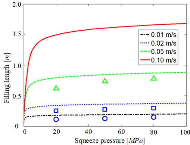
Fig. 8. Comparison of filling lengths between theoretical calculation and experimental measurement of the spiral squeeze casting
