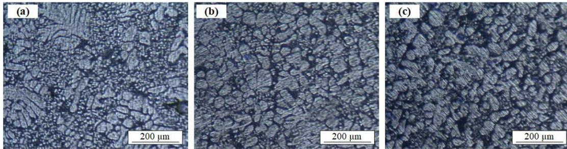
Fig. 3 Microstructure morphology at the filling speed of (a) 0.01 m/s; (2) 0.02 m/s; and (3) 0.05 m/s, respectively.
