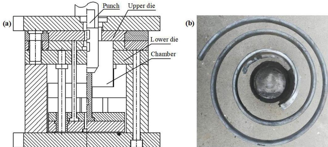
Fig. 1 (a) Self-designed spiral mold structure diagram and (b) spiral specimen.
