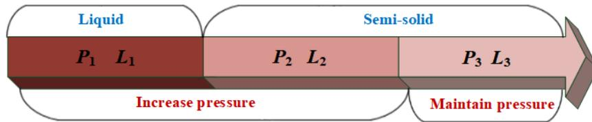
Fig.4 Classification method of pressure loss according to the melt state and filling characteristics.
