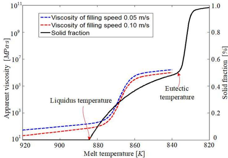
Fig.6 Variation of apparent viscosity and solid fraction with decreasing melt temperature at different filling speeds.
