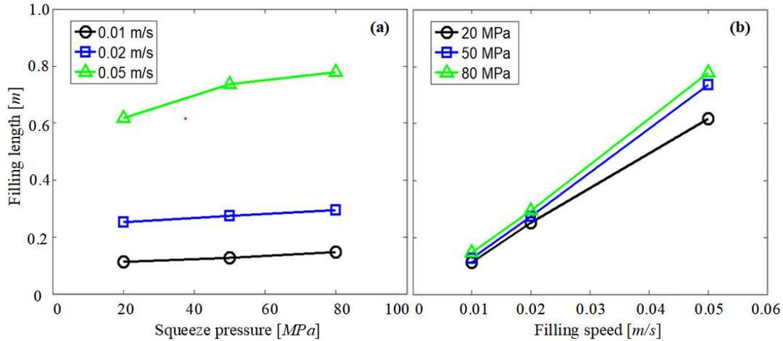
Fig. 2 Variation of filling length with (a) squeeze pressure and (b) filling speed.
