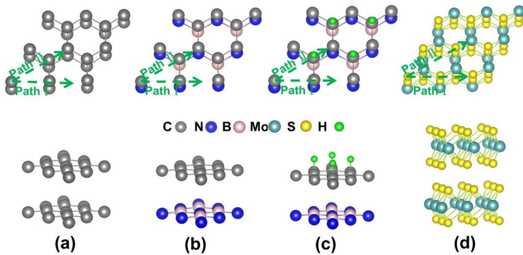
Fig. S1. The sliding models for (a) graphene/graphene, (b) graphene/*h*-BN, (c) H-graphene/*h*-BN and (d) MoS<sub>2</sub>/MoS<sub>2</sub>. The upper and bottom planes are top and side views of bilayer sliding systems, respectively.
