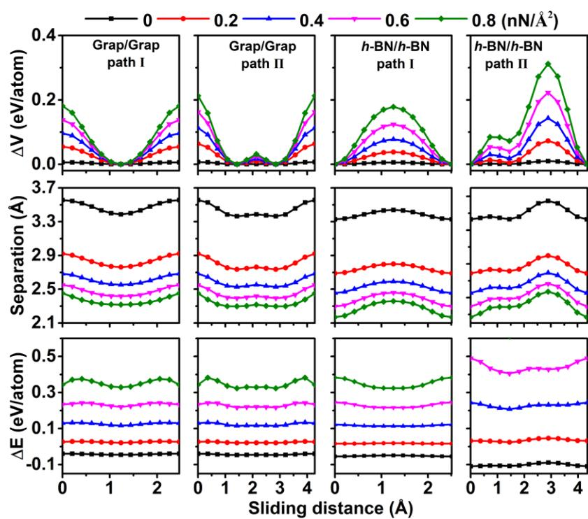
Fig. S5. Sliding barrier  $\Delta V$ , interlayer separation, and binding energy  $\Delta E$  as a function of sliding distance for graphene/graphene and *h*-BN/*h*-BN systems along path I and II, respectively.
