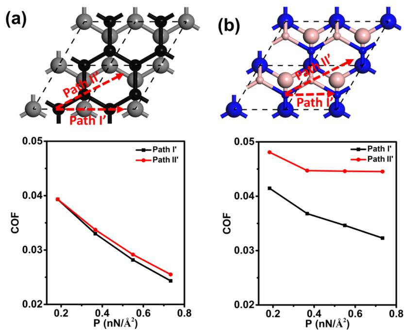
Fig. S2. The structures and friction for (a) graphene/graphene and (b) *h*-BN/*h*-BN systems along two paths with small friction. By moving the two sheets relative to each other by half a bond length, two other small barrier sliding paths were construct. Although the friction and polarity are significantly reduced, the friction difference between the polar and non-polar systems is noticeable.
