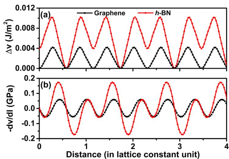
Fig. S3. The comparison of (a) potential barriers and (b) friction forces per unit area along minimum potential energy paths (zigzag path) between graphene/graphene and *h*-BN/*h*-BN systems. The magnitude of barrier in the polar *h*-BN/*h*-BN system is twice that of the graphene/graphene system, and there is a saddle point between two minimum points in the *h*-BN/*h*-BN system.
