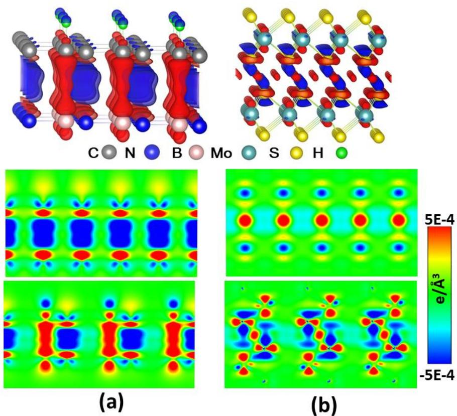
Fig. S6. The charge density difference of (a) H-graphene/*h*-BN and (b) MoS<sub>2</sub>/MoS<sub>2</sub> systems, respectively. Red and blue indicating charge accumulation and depletion regions, and the isosurface charge density is taken as 0.0005 electrons/Å<sup>3</sup>. Middle and bottom planes are the charge density differences along paths I and II shown in Fig. S1.
