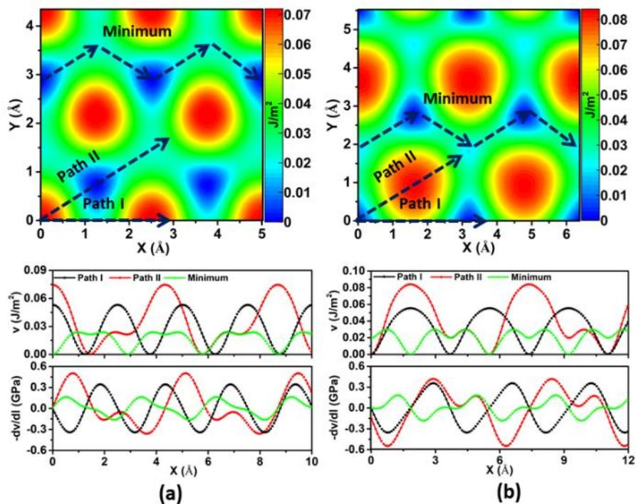
Fig. S4. The potential energy surfaces of (a) H-graphene/*h*-BN and (b) MoS<sub>2</sub>/MoS<sub>2</sub> systems. The absolute PES minimum is taken as a reference. The corresponding potential barriers and friction forces per unit area along the three chosen paths are plotted under each PES.
