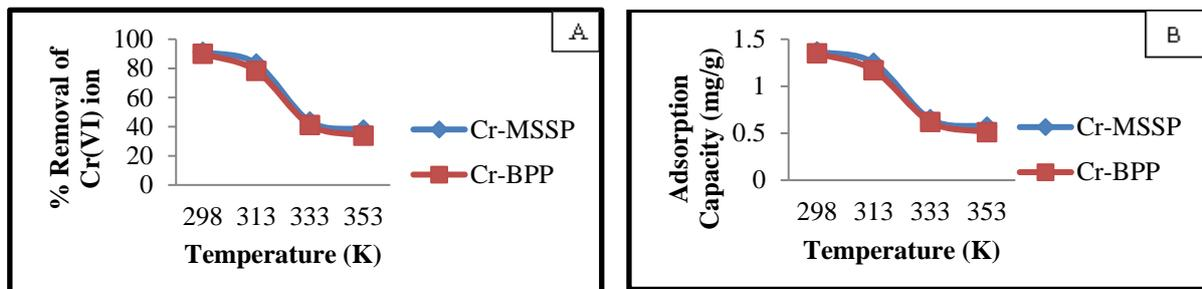
Figure 3.6. Effect of temperature on: a/ % removal of Cr(VI) and b/ adsorption capacity of MSSP (Concentration 30mg/L, dose 20 g/L, contact time 120 min. and pH 2 for Cr(VI) by MSSP and pH 4 for Cr(VI) by BPP).
