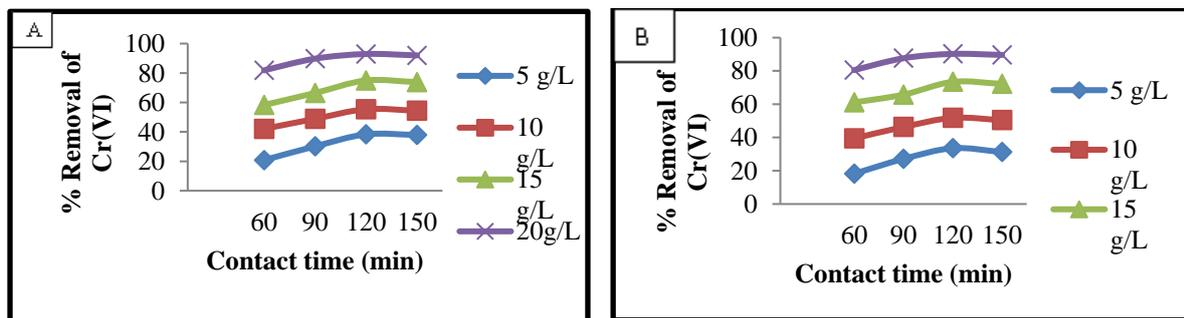
Figure 3.2. Effect of contact time on % removal of: A/ Cr(VI) by MSSP and B/ Cr(VI) by BPP (concentration 30mg/L, contact time 60, 90, 120 & 150 minutes, adsorbent dose 5, 10, 15 & 20 g/L solution, agitation speed 150 rpm and pH = 2 for MSSP, pH = 4 for BPP)
