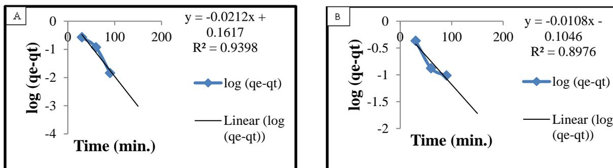
Figure 3.9 Pseudo-first order kinetics plot for A/ chromium by MSSP and B/ chromium by BPP
