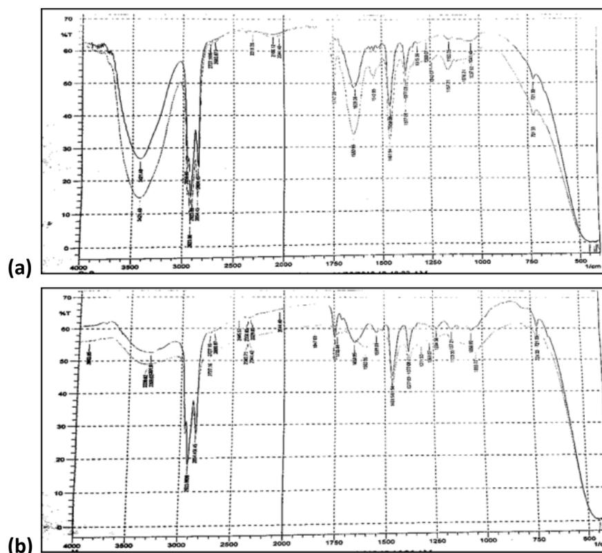
Figure 3.1 FT-IR Spectra of a) BPP and MSSP Before adsorption b) BPP and MSSP after adsorption
