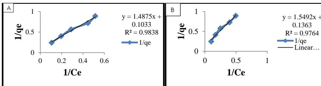
Figure 3.7 Langmuir adsorption isotherms for: A/ Chromium by MSSP and B/ Chromium by BPP.
