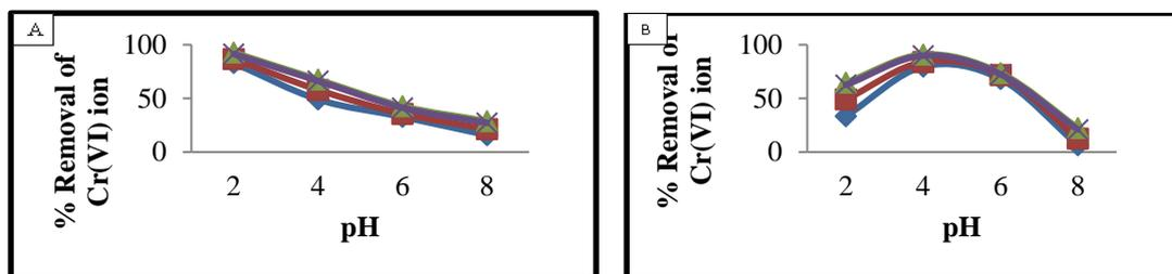
Figure 3.3. Effect of solution pH on % removal of: a/ Cr(VI) by MSSP and b/ Cr(VI) by BPP (concentration 30mg/L, pH, 2, 4, 6 & 8 and contact time 60, 90, 120 & 150 minutes, agitation speed 150 rpm)
