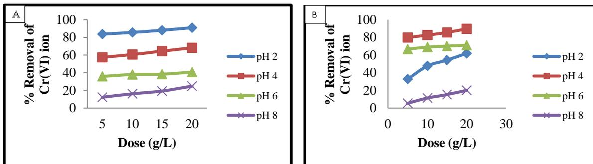
Figure 3.4. Effect of adsorbent dose on % removal of: a/ Cr(VI) by MSSP and b/ Cr(VI) by BPP (concentration 30 mg/L, agitation speed rpm, adsorbent dose 5, 10, 15 and 20 g/L solution, pH 2, 4, 6 & 8).
