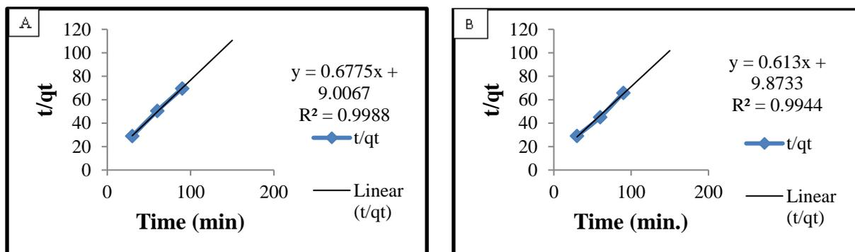
Figure 3.10 Pseudo-second order kinetics plot for A/ chromium by MSSP and B/ chromium by BPP
