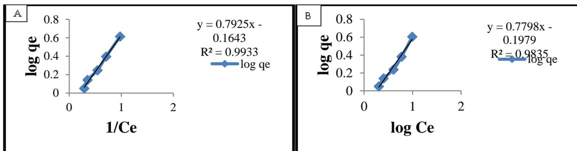
Figure 3.8 Freundlich adsorption isotherms for: A/ Chromium by MSSP and B/ Chromium by BPP
