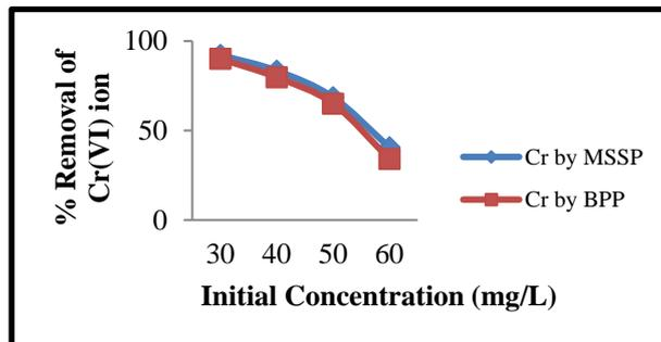
Figure 3.5. Effect of initial concentration on % removal of Cr (VI) by MSSP and by BPP. (dose 20 g/L, contact time 120 min. and pH 2 for Cr(VI) by MSSP and pH 4 for Cr(VI) by BPP)
