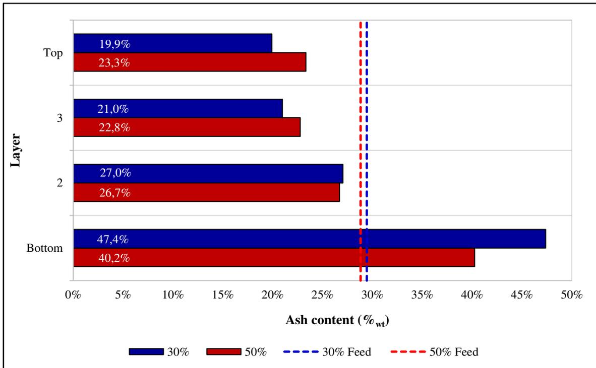
**Figure 8: Ash analyses for +4.75-5.6mm particles at 21.97 Hz**
