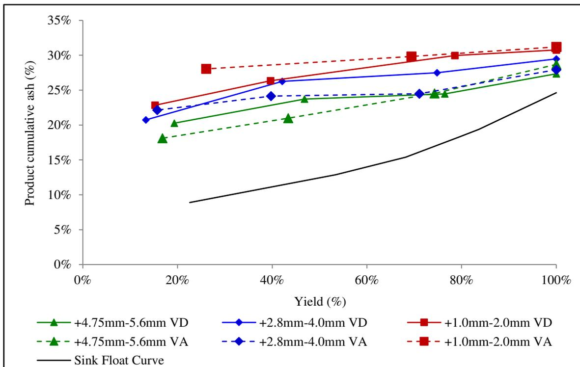
**Figure 3: Comparison of bed performance curves for various PSD's (DM 0:1; VD and VA)**
