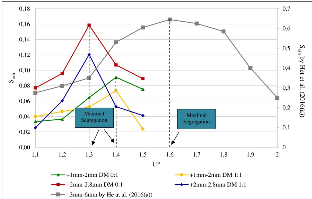
**Figure 6: Degree of segregation for PSD-02 and PSD-03 compared to the segregation degree adapted from He *et al.* (2016(a)).**
