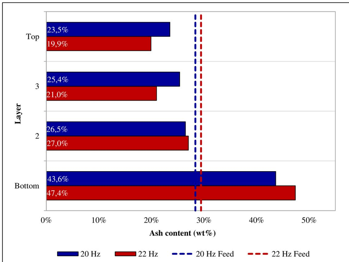
**Figure 7: Ash analyses for +4.75-5.6mm particles and 30% amplitude and 20 Hz**
