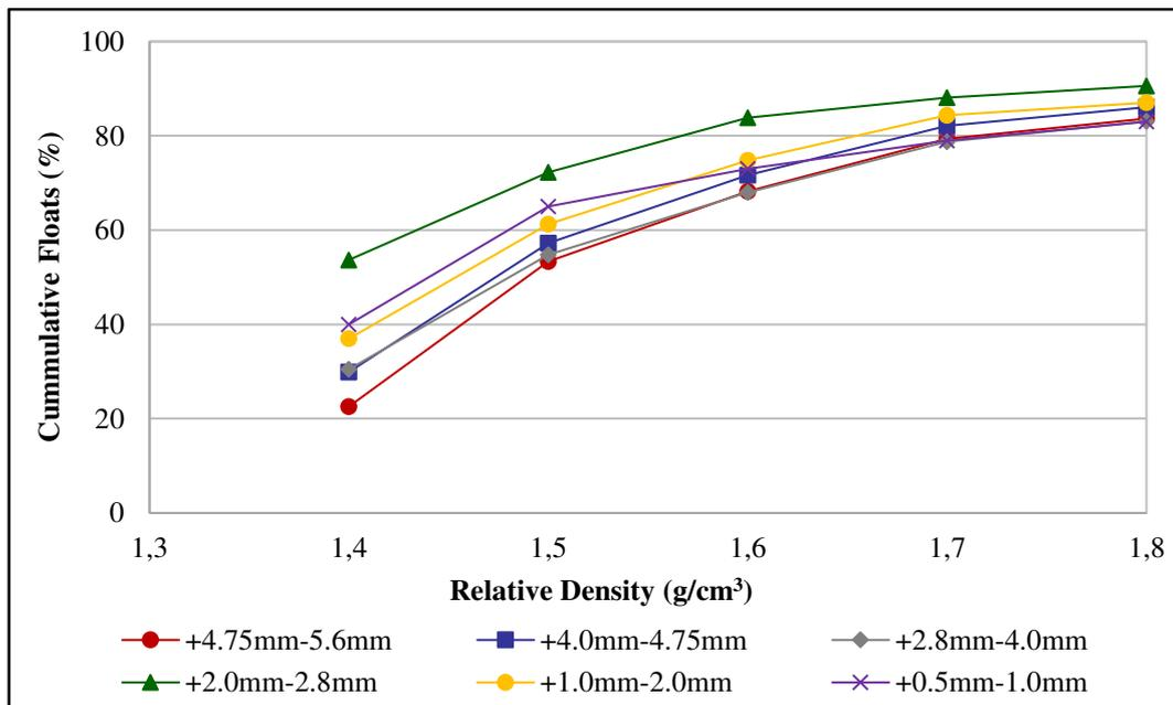
Figure 1: Density profiles for +0.5mm-5.6mm coal
