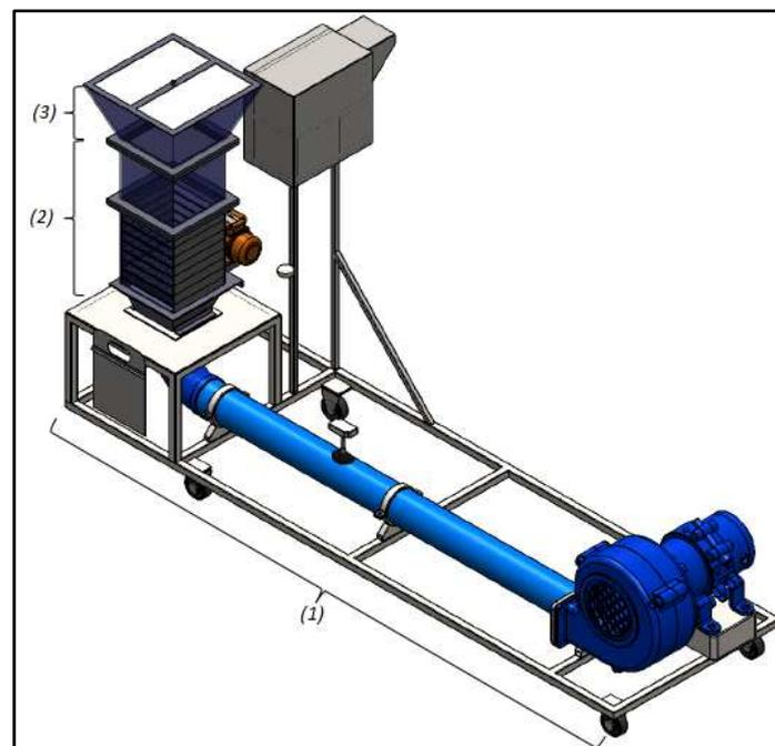
**Figure 2: Three-dimensional illustration of the ADMFB with (1) airflow system, (2) fluidized bed system and (3) dust control section**
