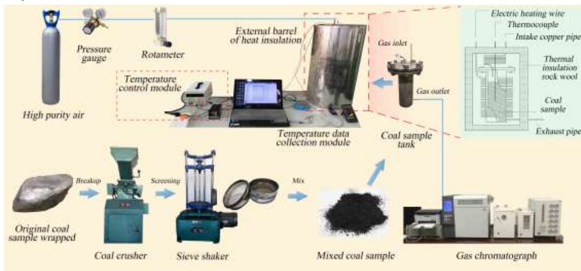
Figure 1 Temperature-programmed experimental system for coal oxidation
