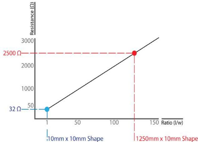
**Figure 1.** Resistance graph of the relationship between length/width ratio and resistivity.
