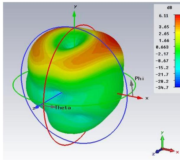
**Figure 8.** Gain change depending on the angle value of the designed antenna for conductive paint.
