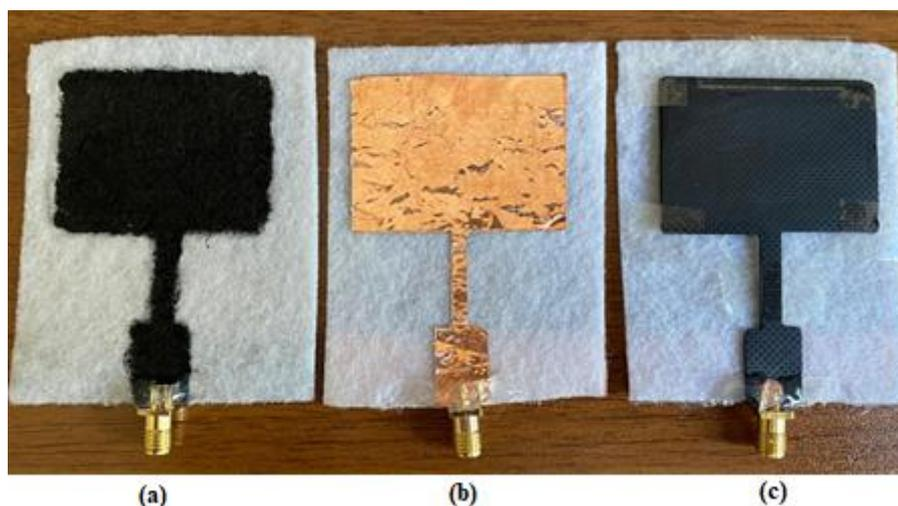
**Figure 5.** The manufactured antennas: (a) Conductive Paint, (b) Copper Tape, and (c) Graphene antenna with a felt substrate.
