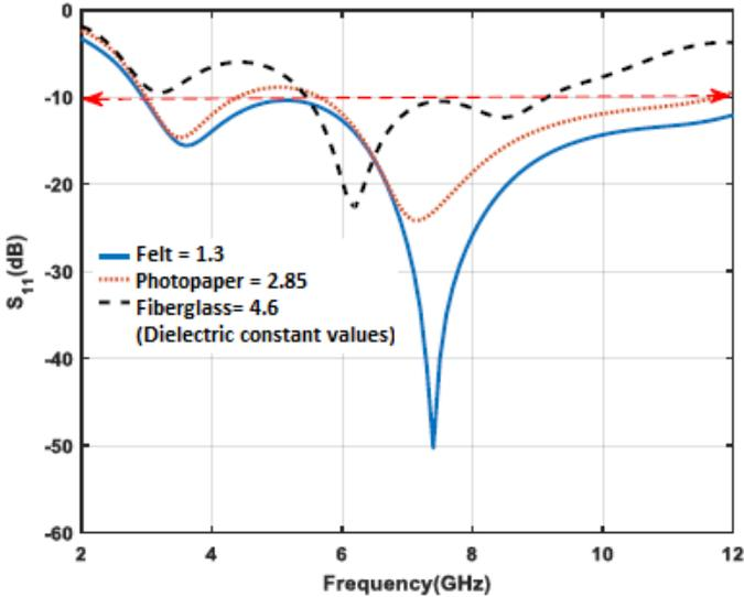
Figure 3. Comparison of the substrates with different dielectric constants in the simulation environment.
