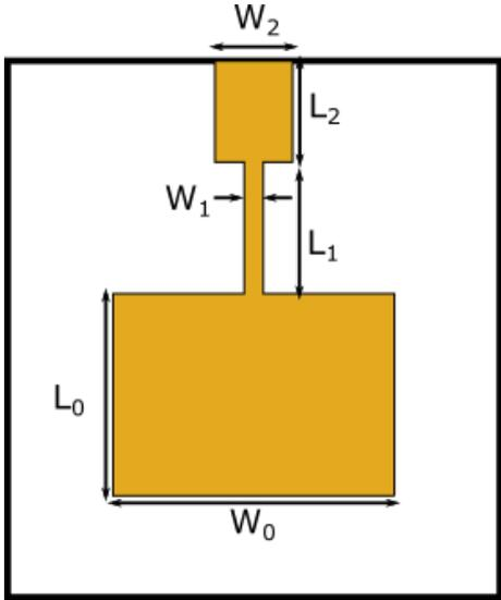
Figure 2. Proposed antenna structure.
