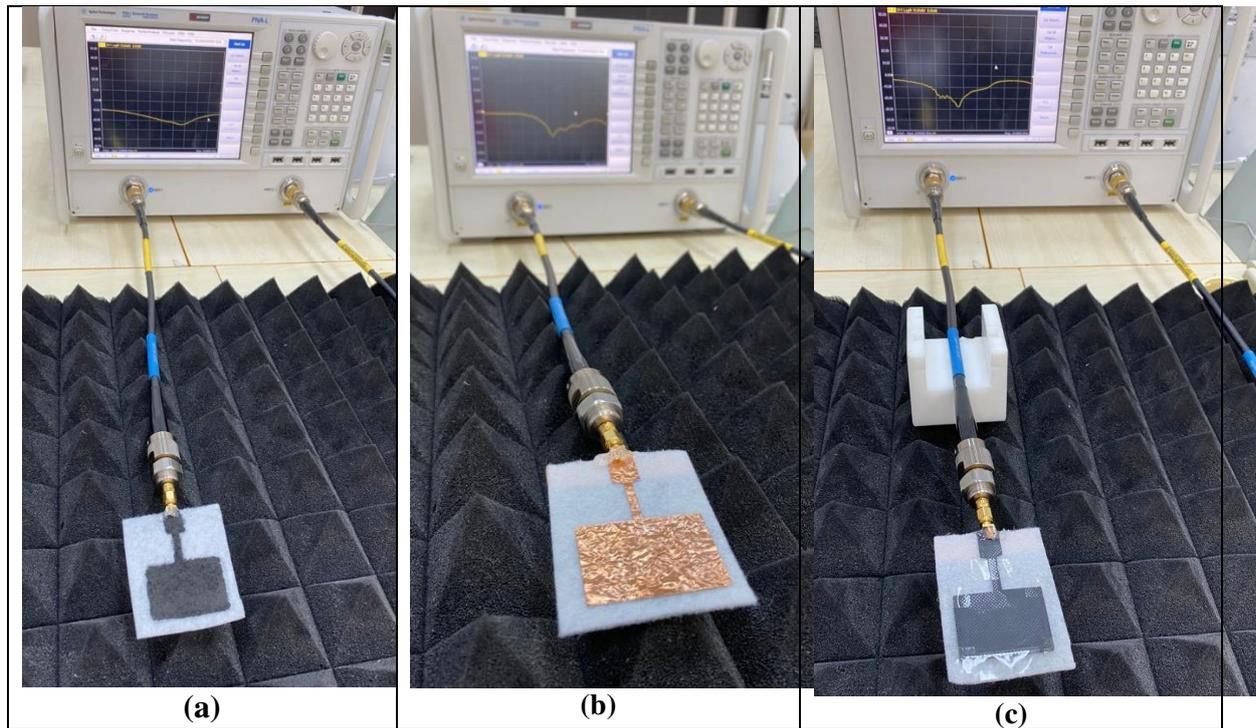
**Figure 6.** Measurement setup: (a) Conductive Paint, (b) Copper Tape, and (c) Graphene antenna with felt substrates.
