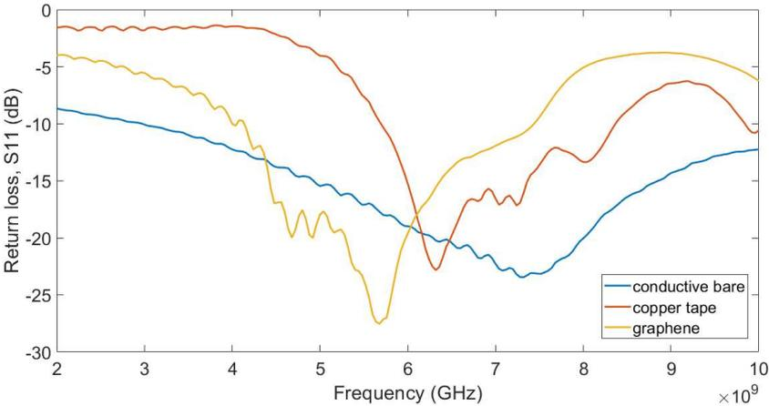
**Figure 7.** Comparison of measured return loss values for copper tape, graphene, and conductive bare, respectively.
