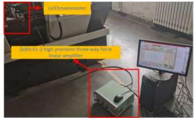
Fig. 2 Schematic diagram of force measuring system
