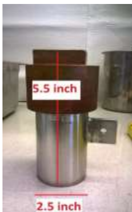
126 Fig. 2.d – MDOB - Dimensions of the digesters
