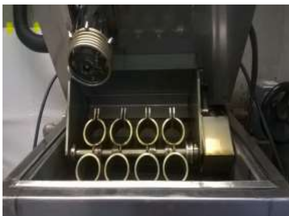
122 Fig. 2.b - MDOB – Clamps for holding the digesters and heat exchanger coil
