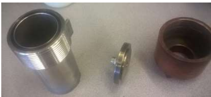
124 Fig. 2.c - MDOB – Digester, lid, and brass cover
