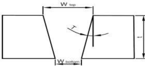
Fig. 4. Abrasive water jet cut profile
