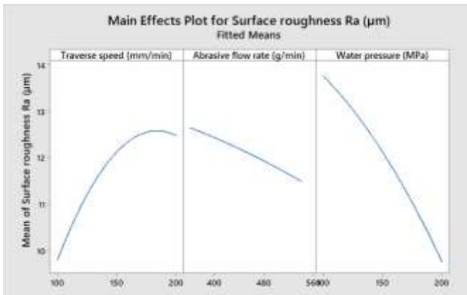
Fig. 7. Variation process parameters with mean of surface roughness
