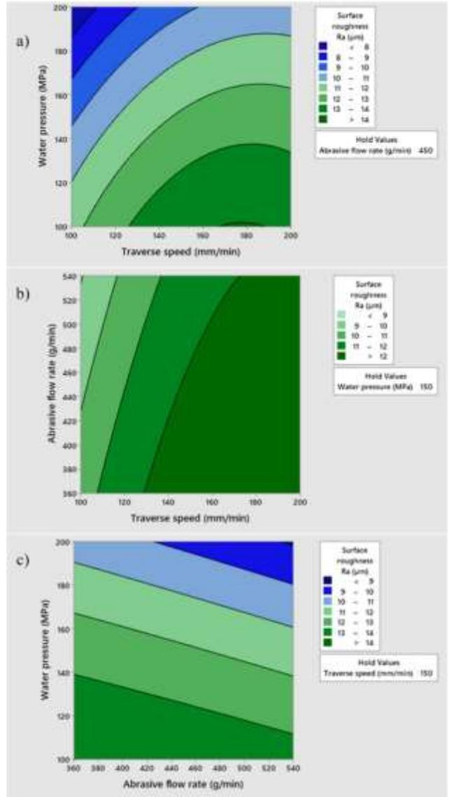
Fig. 8 Contour plot of surface roughness with a) water pressure and traverse speed , b) abrasive flow rate and traverse speed, and c) water pressure and abrasive flow rate.
