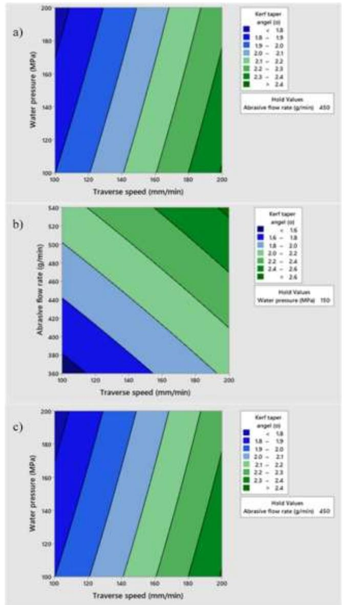
Fig. 10 Contour plot of kerf taper angle with a) water pressure and traverse speed, b) abrasive flow rate and traverse speed, and c) water pressure and abrasive flow rate.
