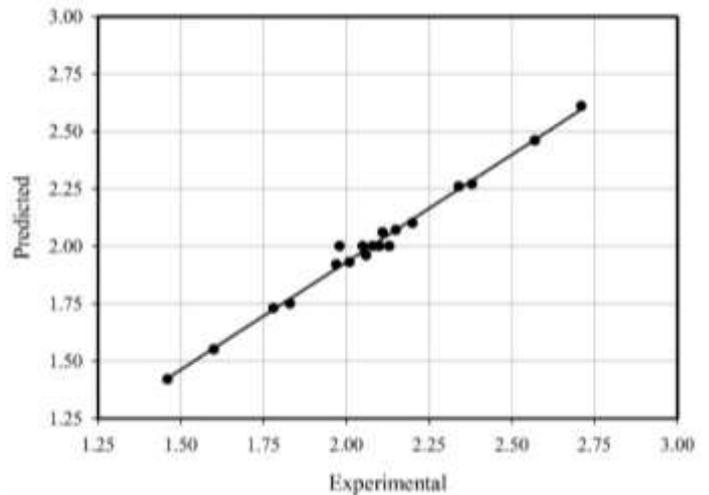
**Fig. 6.** Comparison of predicted kerf taper angle with experimental measurements
