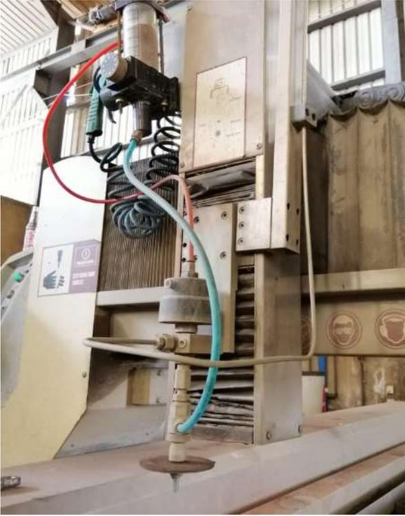
Fig.1. Abrasive water jet cutting machine.
