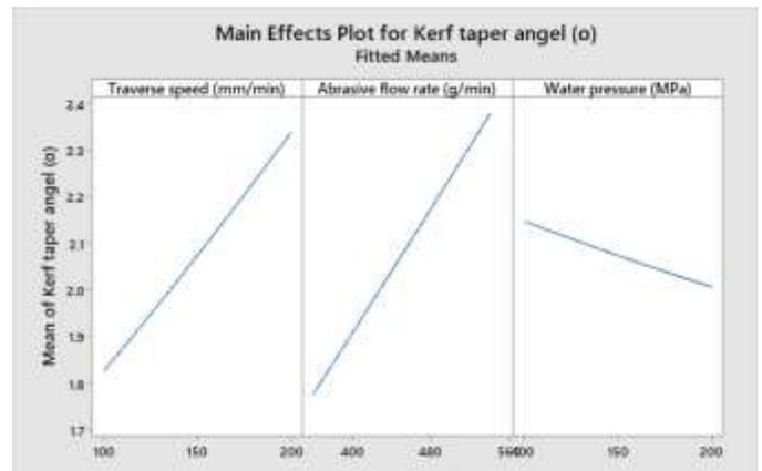
Fig. 9. Variation of process parameters across Kerf taper
