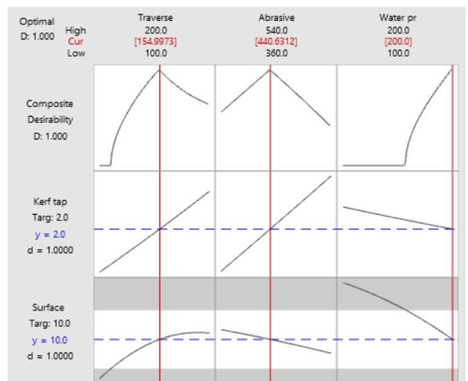
Fig. 11. Validation of quadratic model for surface roughness and kerf taper angle.
