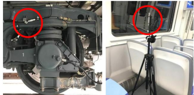
Figure 2 Wheel–rail noise and interior noise measurement
