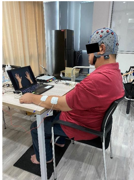
128 Figure 1. The components of AOMI-based BCI with the FES system that the participant was given 129 on each training day. The system was composed of a g. tec biosignal amplifier, computer, and the 130 FES.
