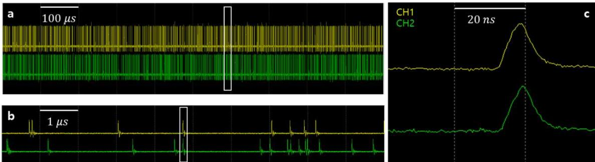
**Fig. 3| Sub-Poisson distributed photon characteristics observed by a fast digital oscilloscope.** **a**, Photon streams detected by D1 (yellow) and D2 (green) in Fig. 1 without BS2. **b**, Expansion of the box in **a**. **c**, Expansion of the box in **b** for a coincident (doubly bunched) photon pair.
