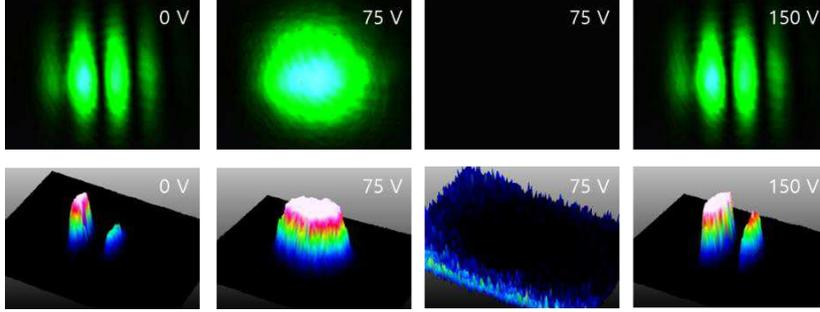
**Fig. 2| One-axis PZT controlled coherence modification (see Fig. 1b).** (Top) 2D images captured on CMOS (see the inset of Fig. 1b). (Bottom) 3D analyses for Top images. The flat top indicates saturated intensity of light.
