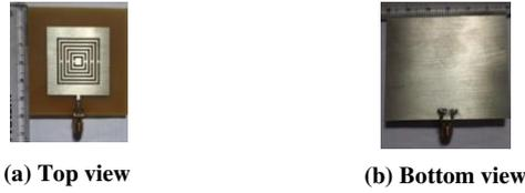
**Fig. 4** Photograph of the fabricated antenna having 6 rings
