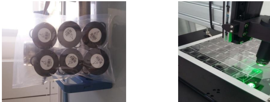
175 176 Figure 4 - Pictures of CR39 devices (left) and the optical microscope Politrack (right)
