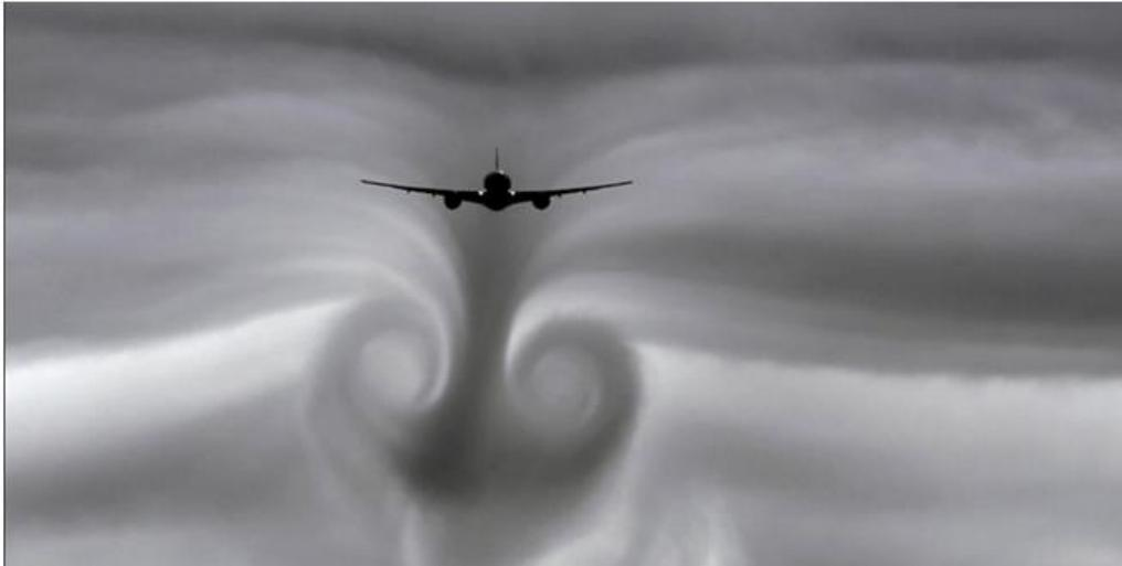
Figure 3. In this photograph, the vortex air movement is clearly visible in the form of two vortices with horizontal axes that follow the two wings of the airplane.
