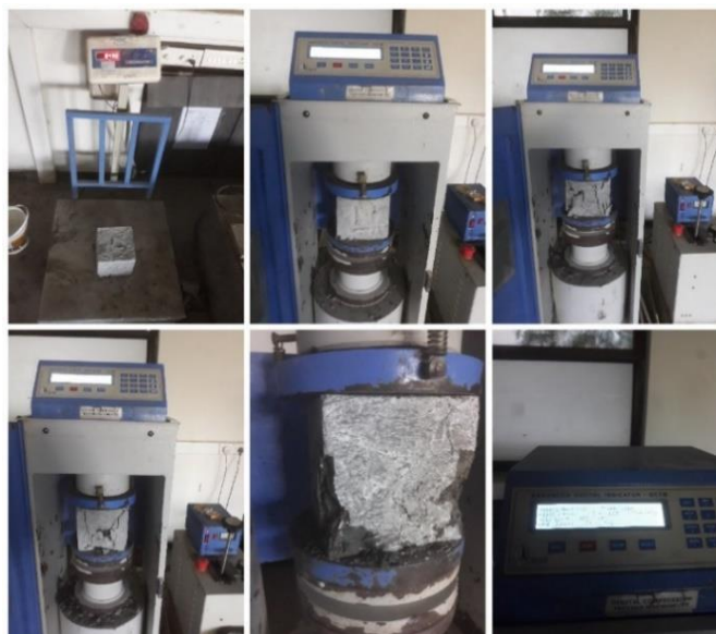
Figure 4. Compressive strength test.
