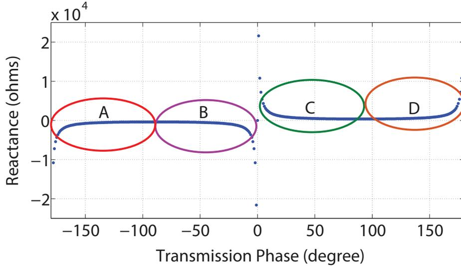
**Figure 2.** The transmission reactance values in terms of the transmission phase under the following assumptions: lossless unit cell ( $|S_{11}| = 0, |S_{12}| = 1$ ), and available phase range =  $360^\circ$ . Apparently,  $A=B$ , and  $C=D$ .
