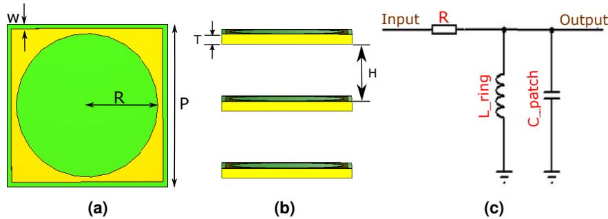
**Figure 3.** The triple layer unit-cell layout of a square ring element and a circular patch. (a) top view, (b) side view, and (c) the equivalent circuit of one layer unit-cell. Note that the green parts represent metal, and the yellow parts represent dielectric.
