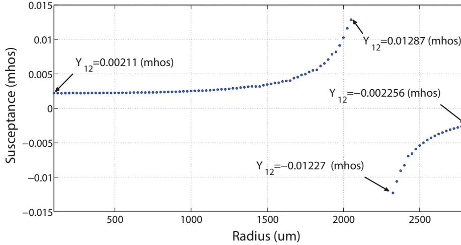
**Figure 5.** Simulated susceptance values in terms of the circular patch radius  $R$  under the normal incident angle at 12 GHz. The bounds are specified with arrows. The maximum susceptance value is 0.01287, and the minimum value equals -0.01227.
