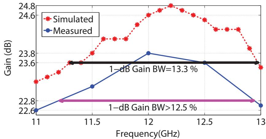
**Figure 9.** The measured and simulated gains versus frequency.
