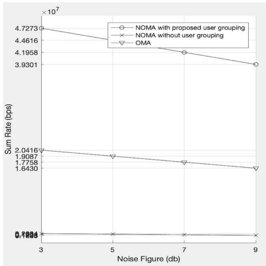
Fig. 6 Comparison of the Proposed Algorithm with OMA and NOMA without user grouping in 20 groups
