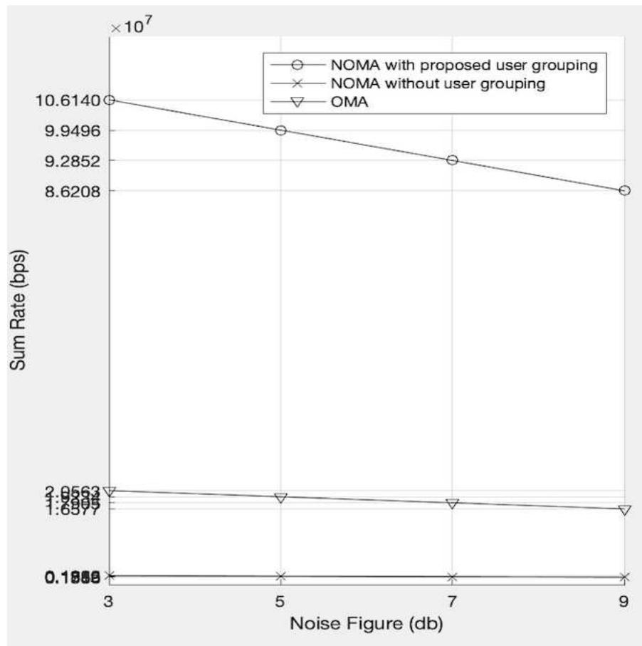
Fig. 7 Comparison of the Proposed Algorithm with OMA and NOMA without user grouping in 50 groups
