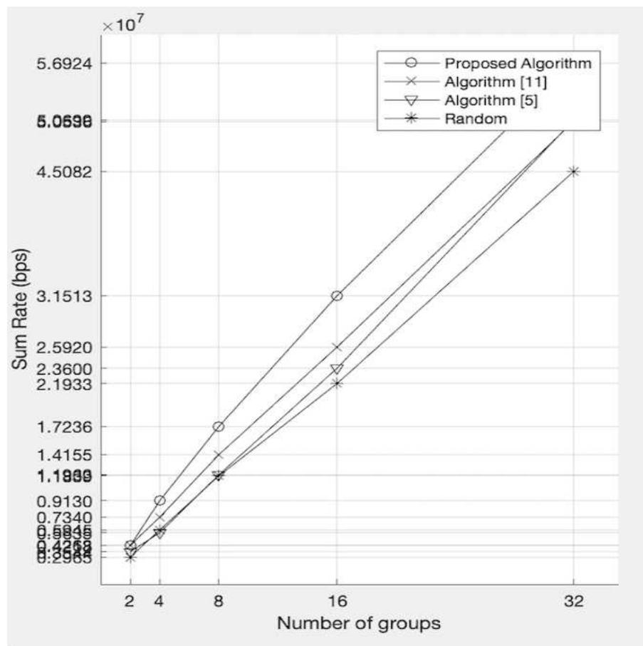
**Fig. 9** Sum-rate comparison of the Proposed Algorithm with random user grouping, algorithm [5] and algorithm [11] with 64 users
