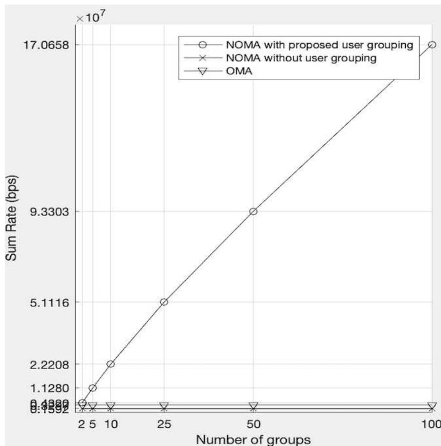
**Fig. 5** Comparison of the Proposed Algorithm with OMA and NOMA without user grouping with 200 users
