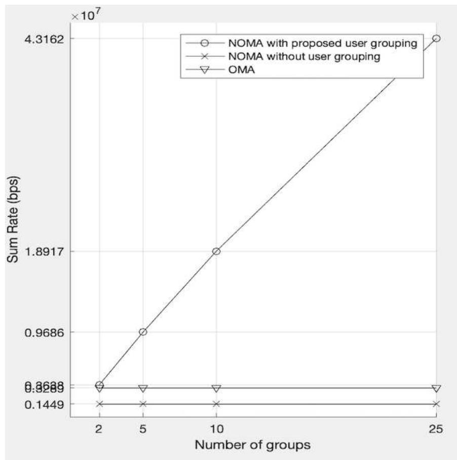
**Fig. 3** Comparison of the Proposed Algorithm with OMA and NOMA without user grouping with 50 users
