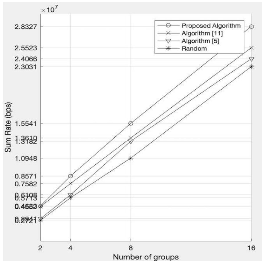
Fig. 8 Sum-rate comparison of the Proposed Algorithm with random user grouping, algorithm [5] and algorithm [11] with 32 users
