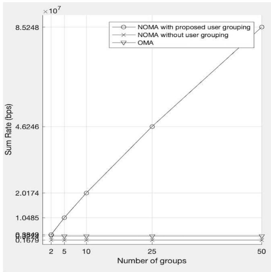
Fig. 4 Comparison of the Proposed Algorithm with OMA and NOMA without user grouping with 100 users
