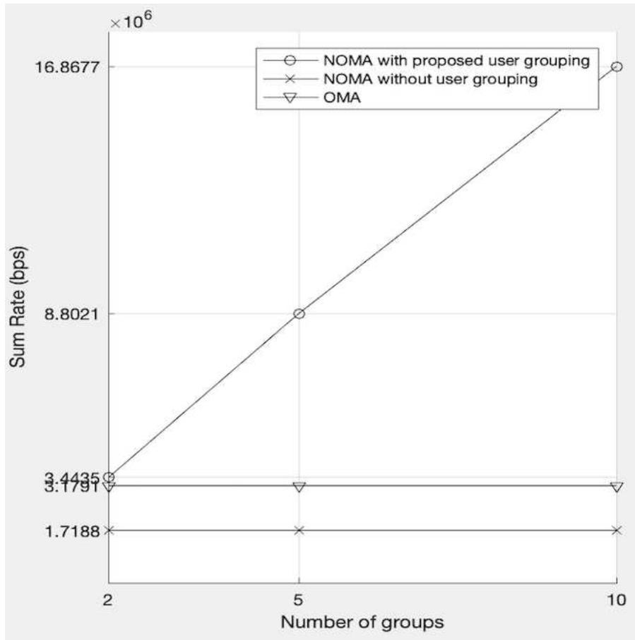
**Fig. 2** Comparison of the Proposed Algorithm with OMA and NOMA without user grouping with 20 users
