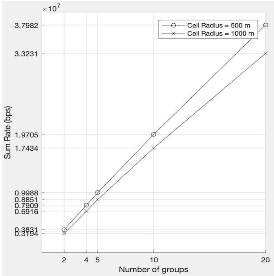
Fig. 13 Sum-rate comparison of the Proposed Algorithm in different cell radius
