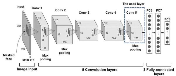
Fig. 5: AlexNet network architecture introduced in [15].
