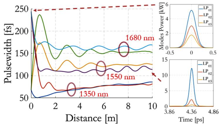
Fig. 3 – Simulated soliton pulse widths for input pulses of 67 fs and 235 fs duration, and input wavelengths of 1350 nm, 1550 nm, 1680 nm, respectively. The input modes are LP<sub>01</sub>, LP<sub>02</sub>, LP<sub>03</sub>. Right insets: modal powers at the fiber input (top), and after 10 m of propagation (bottom), for 1550 nm input wavelength and 235 fs input pulsewidth.
