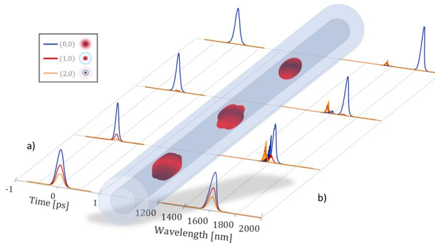
Fig. 2 – Spatiotemporal soliton formed from an input 235 fs pulse, composed by 3 axial modes, propagating over 120 m of GRIN fiber, at an optimal input energy of 2.5 nJ. a): modes power, b): modes spectra.
