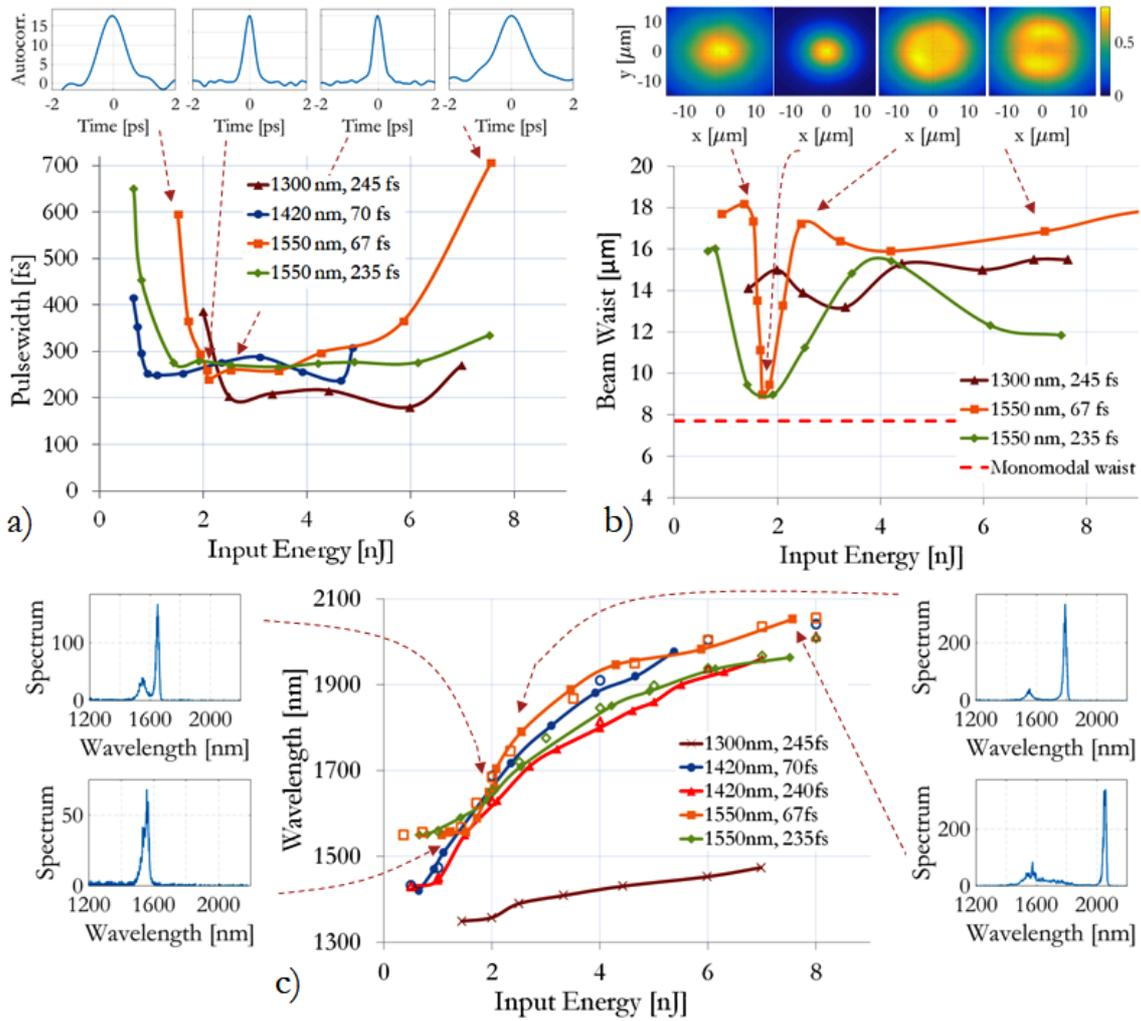
Fig. 1 – Measured soliton pulsewidth (a), beam waist (b), and wavelength (c) vs. input pulse energy, after 120 m of GRIN fiber, for different input wavelengths and pulse durations. The insets are the measured autocorrelation traces (a), output near-fields (b), and spectra (c), for input wavelength 1550 nm and pulsewidth 67 fs.
