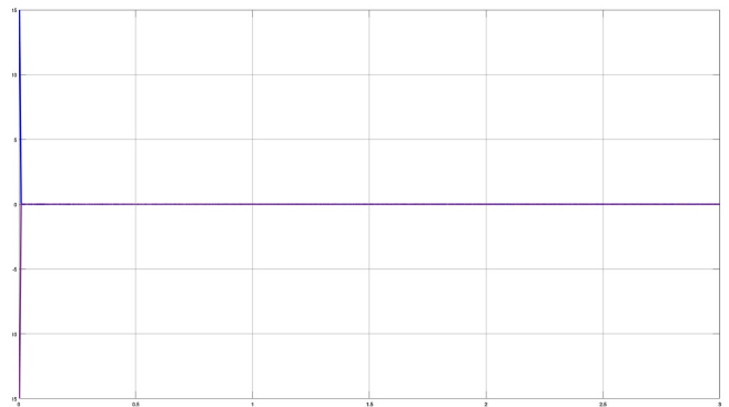
Fig. 5 Sliding variables s_t converging to zero.
