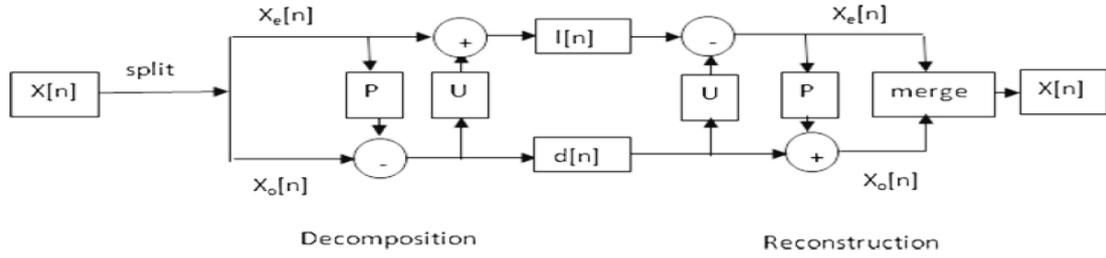
Figure 1. Decomposition and Reconstruction of a signal  $X[n]$  using  $LWT$  and its inverse respectively.
