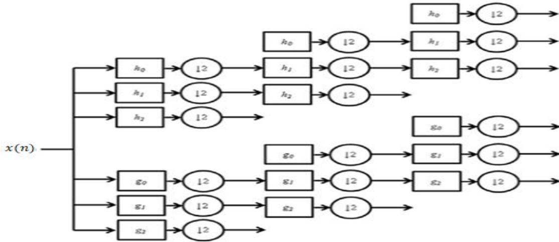
Figure 3. Filter bank diagram of 1 –  $D$  double density complex  $DWT$ .
