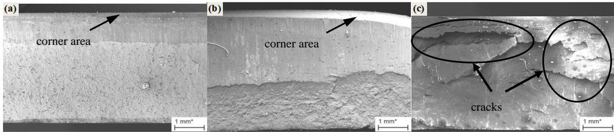
**Fig. 2.** Comparison of typical sheared edge profiles obtained at room temperature: (a)Q235 steel, (b) aluminum alloy, (c) as-cast AZ31 magnesium alloy.
