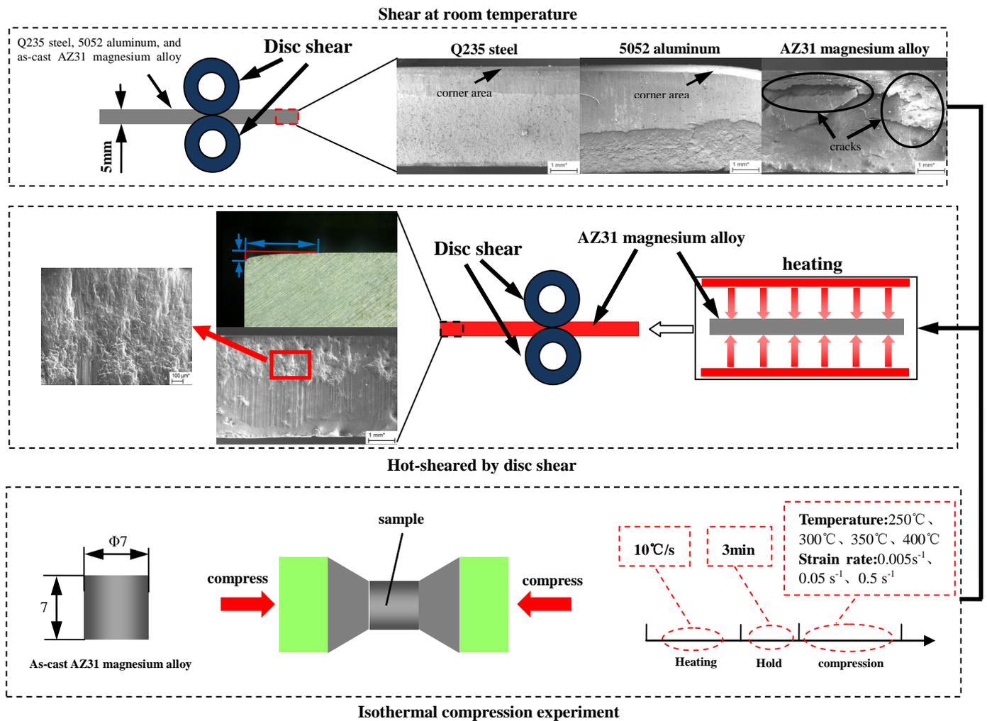
Fig. 1. Schematic diagram of the Shear experimental
