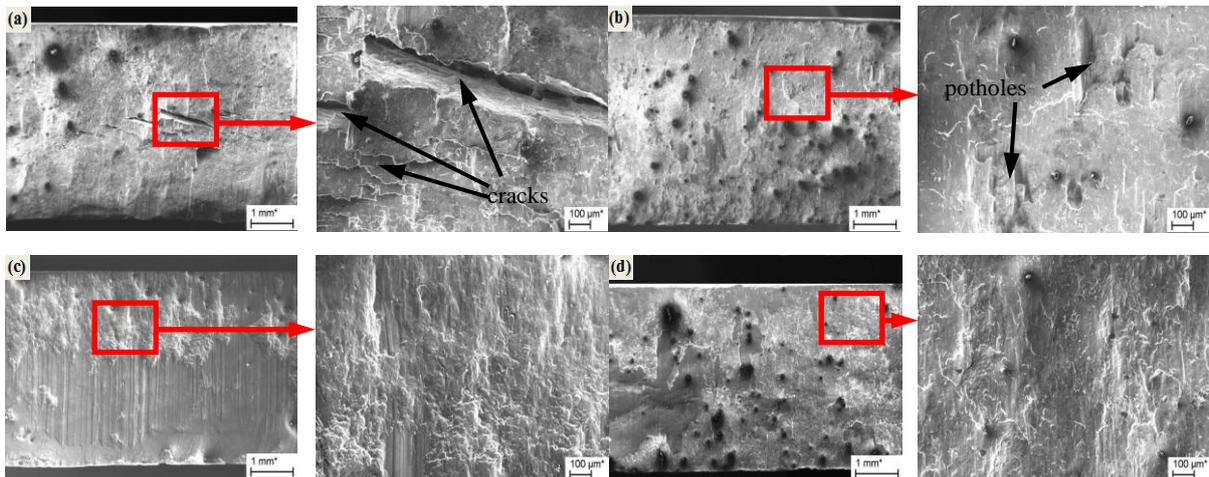
**Fig. 4.** Comparison of typical sheared edge profiles obtained at different temperature of AZ31 magnesium alloy: (a)100 °C, (b)200 °C, (c) (c)300 °C, (d)400 °C
