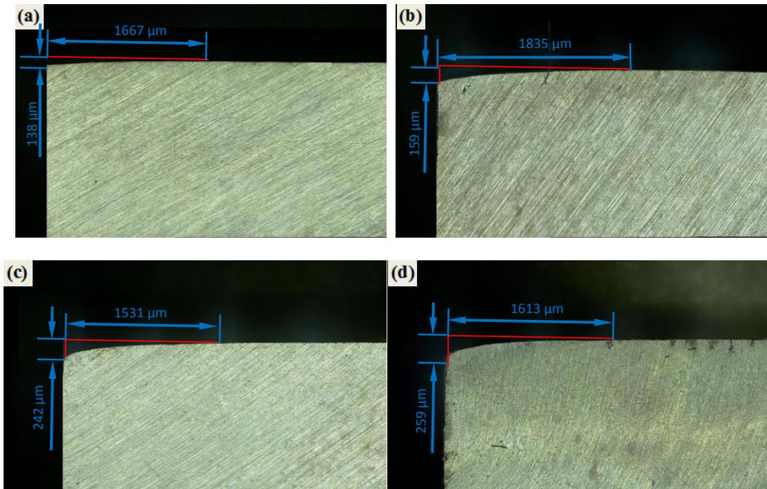
**Fig. 3.** Comparison of Fillet area obtained at different temperature of AZ31 magnesium alloy: (a)100°C, (b)200°C, (c)300°C, (d)400°C
