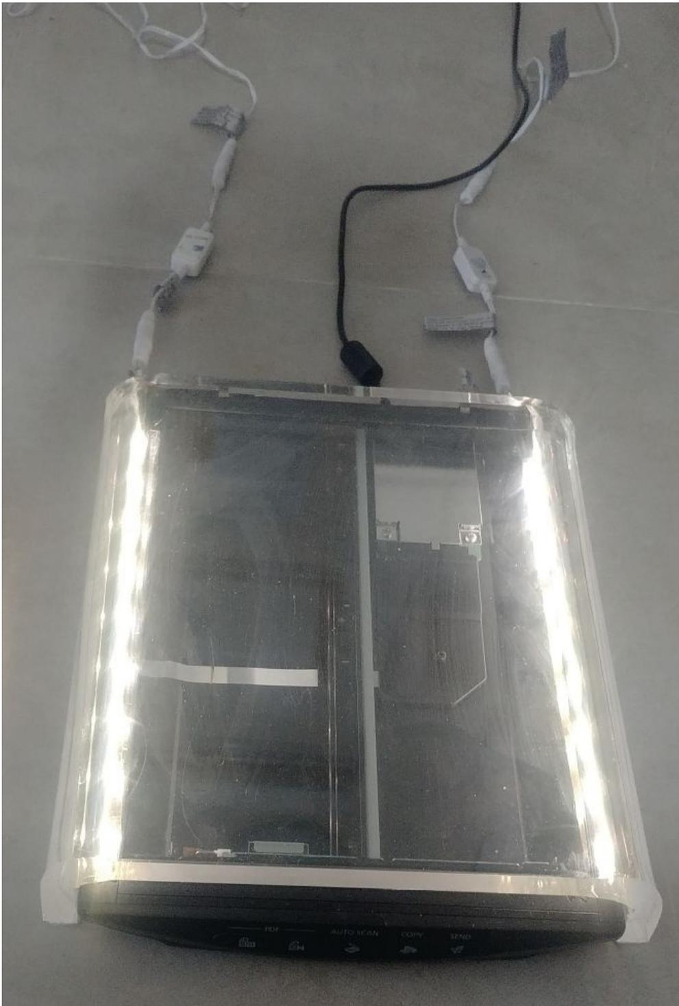
**Fig.7 System for detection of feet during standing**
