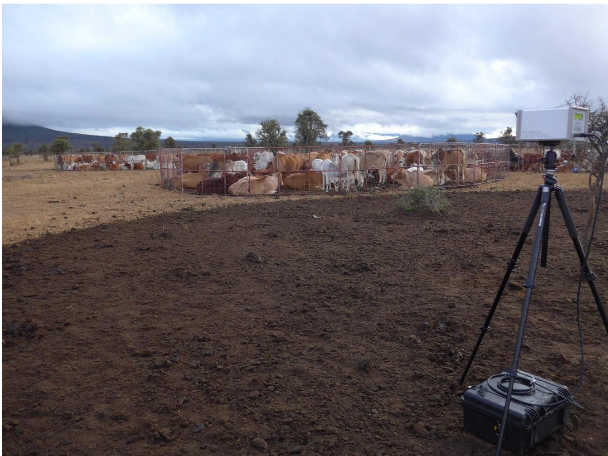
184 Fig. 2 Typical field setup, with one of the laser spectrometers on the right-hand side and bomas in the background
