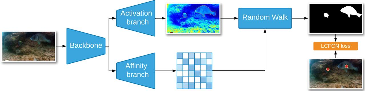
**Figure 3. Affinity-based architecture.** The first component is the ResNet-38 backbone which is used to extract features from the input image. The second component is the activation branch outputs per-pixel scores. The third component is the affinity branch outputs an affinity matrix. These two outputs are aggregated using a random walk to get the final, refined per-pixel output.
