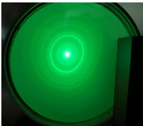
**Figure 3.** The influence of the magnetic field on the electron diffraction pattern.
