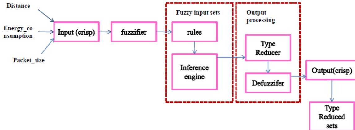
Figure 8 Block diagram of Type2 fuzzy-based recovery system
