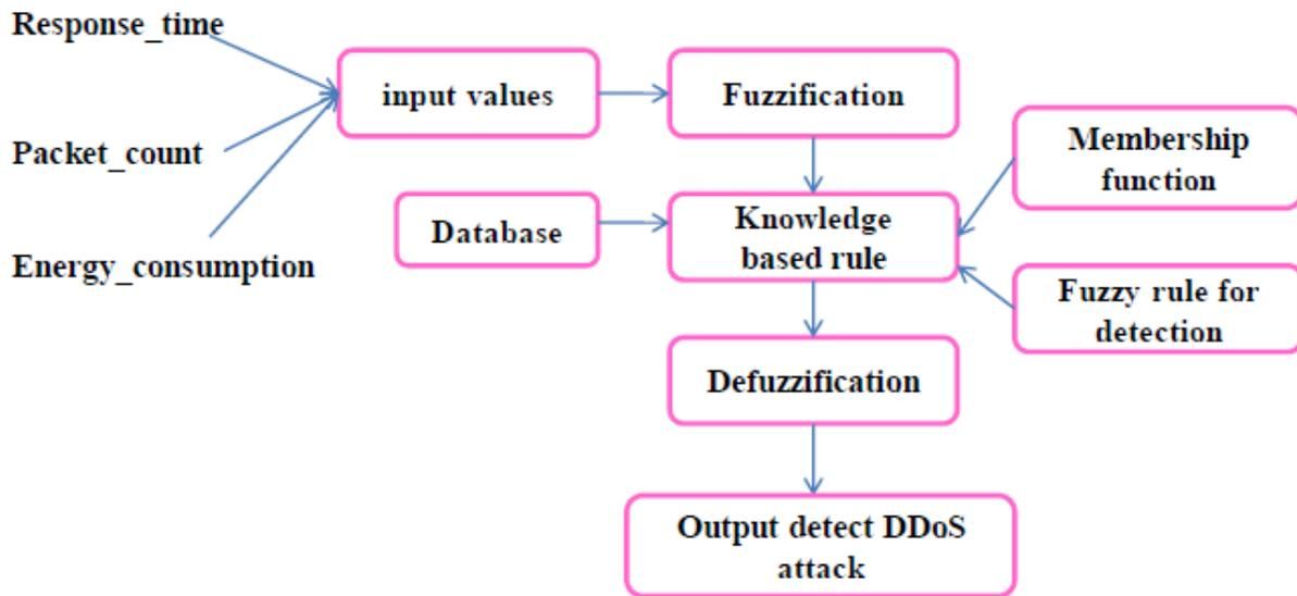
Figure 2. Type1 Fuzzy based DDoS attack detection system
