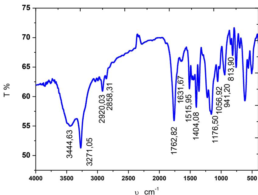
**Fig 3. FTIR spectrum of alkalized *Luffa Cylindrica* (LC) biosorbent**
