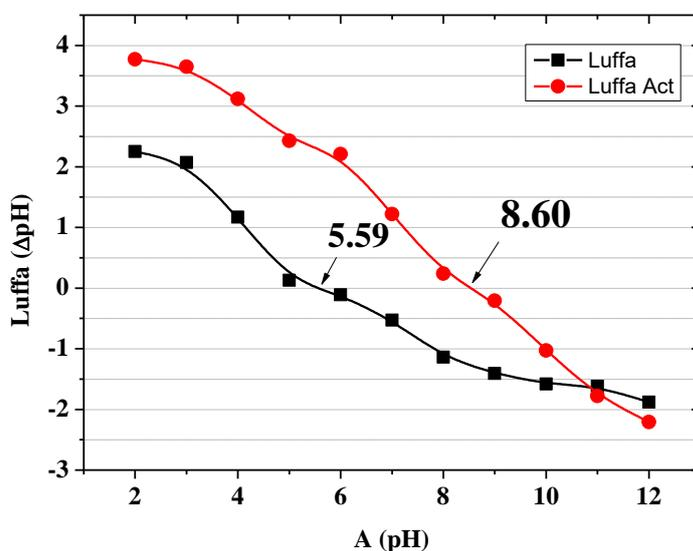
**Figure S1:** pH of zero charges of natural and modified *luffa*
