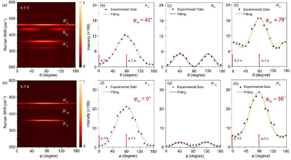
**Fig. 2** ARP Raman scattering spectra of BP for (a)-(d) basal plane and (e)-(h) cross plane. ARP Raman scattering intensities were fitted with Eq. (4) and (6), and the phase differences between Raman tensor elements  $a$  and  $c$   $\phi_{ac}$  of  $A_g^1$  and  $A_g^2$  modes are  $42^\circ$  and  $79^\circ$  for basal plane. For cross plane, the phase differences between Raman tensor elements  $b$  and  $c$  of  $A_g^1$  and  $A_g^2$  modes are  $0^\circ$  and  $50^\circ$  respectively.
