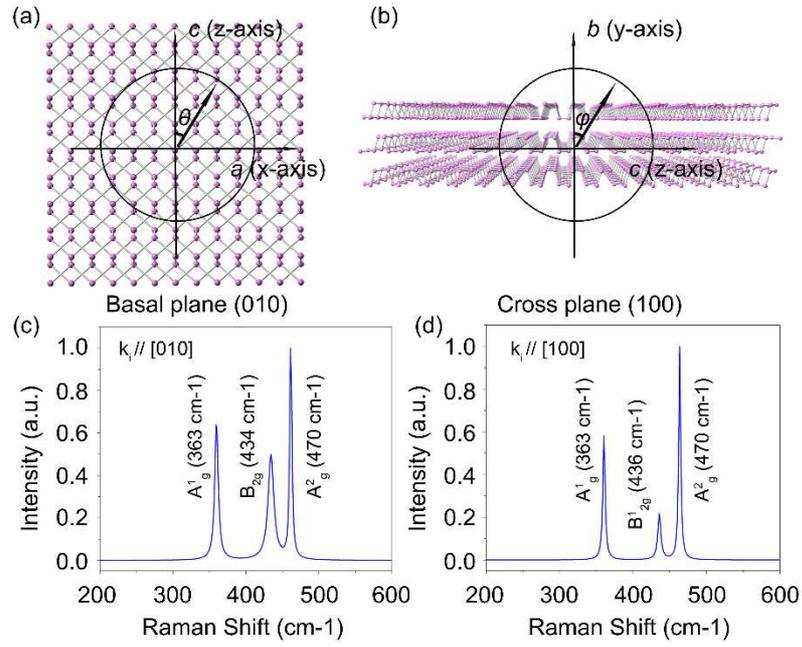
**Fig. 1** Schematic of ARP Raman scattering of basal and cross plane of BP. (a) ARP Raman scattering of basal plane,  $\theta$  is the angle between polarization direction of incident light and  $c$  axis. (b) APR scattering of cross plane,  $\varphi$  is the angle between polarization direction of incident light and  $b$  axis. (c) and (d) denote representative Raman spectra of basal and cross plane.
