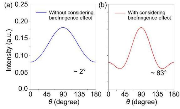
**FIG. 3** Calculated basal plane APR spectrum of  $A_g^2$  with and without considering birefringence effect.
