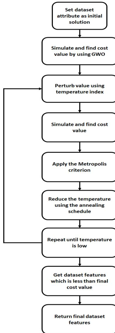
Fig. 2 Proposed Enhanced simulated annealing work flow
