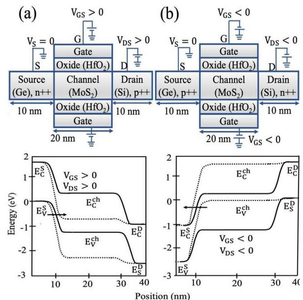
Fig. 1. Schematic diagram and the corresponding band diagrams of (a) n-type TFET, (b) p-type TFET at both off (lines) and on (dotted) state. Arrow direction indicates the direction of carrier flow.
