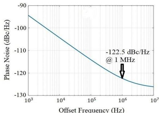
Fig. 8. Simulated phase noise of the ring oscillator.
