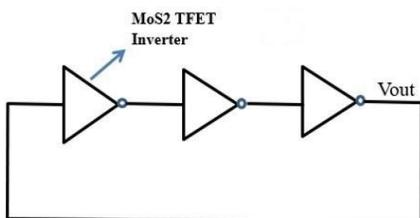
Fig. 6. Diagram of three stage MoS<sub>2</sub> TFET ring oscillator.
