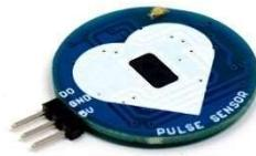
**Figure 5:** Pulse Sensor
