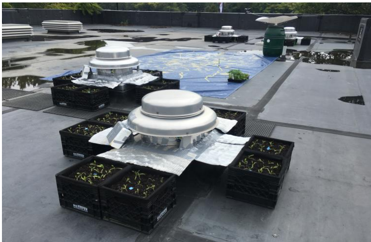
Figure 1. Experimental garden set up around rooftop exhaust vents and control fans. Spinach and corn were planted in milk crates provided by Recover Green Roofs positioned next to various vents for four and a half weeks until harvest after which growth was measured.
