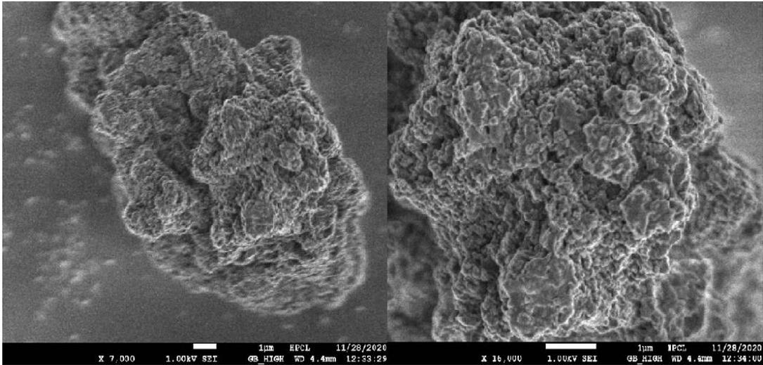
Fig.2 SEM images of alkali treated lignin at magnifications 7000 X, 16000X
