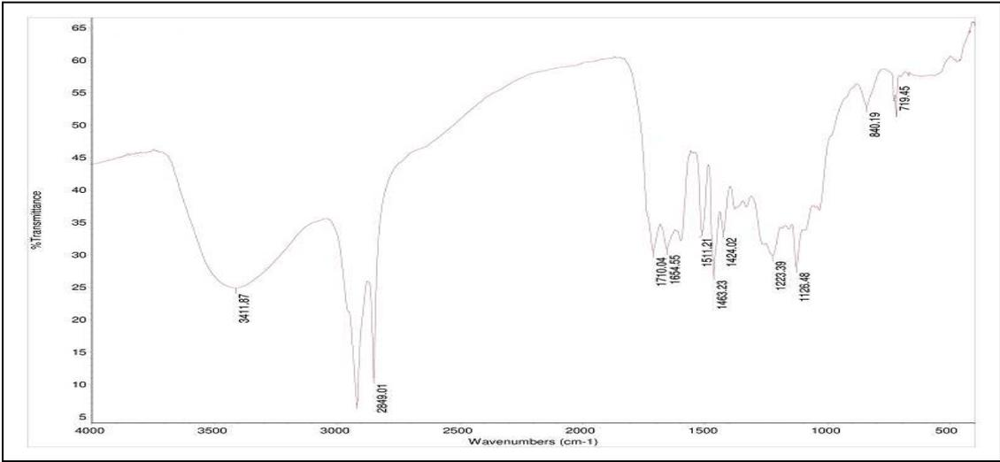
Fig.1 FTIR spectra of alkali lignin
