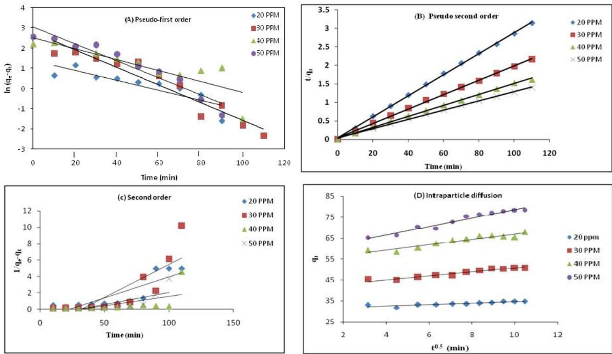
Fig.9. The kinetic models for adsorption of MG onto lignin
