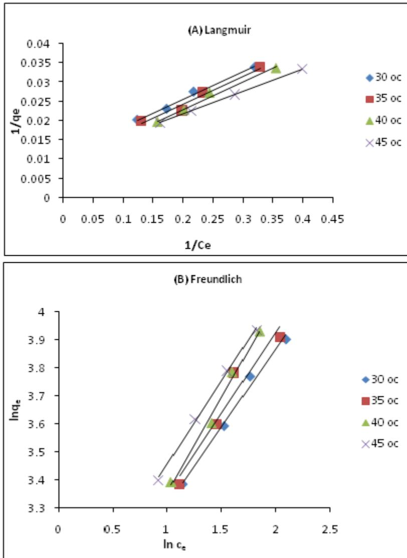
Fig.10 The isotherm models for adsorption of MG onto lignin
