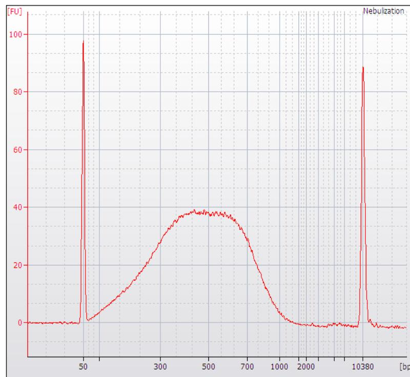
Figure 4: DNA 7500 LabChip profile of a nebulized and purified DNA sample for use in the preparation of a GS Junior Titanium Paired End library
