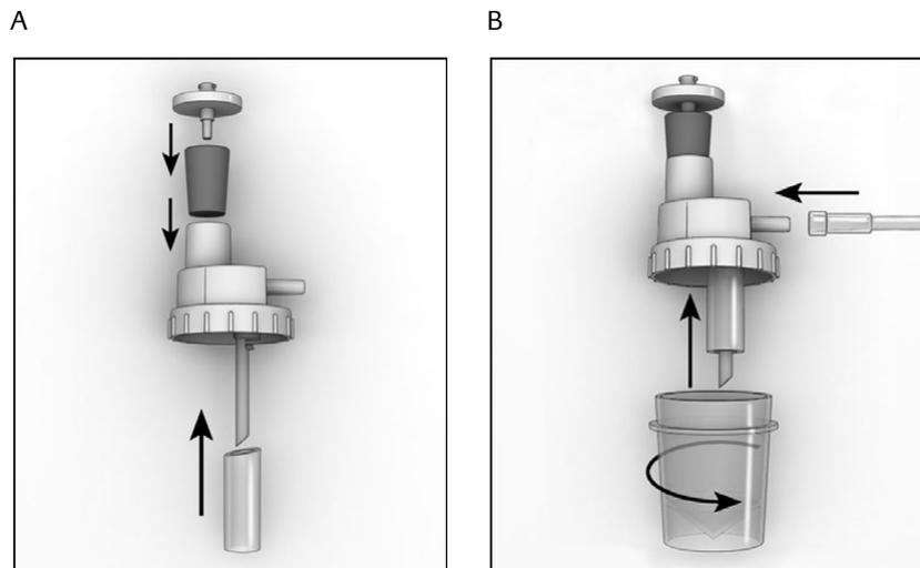
Figure 2: Assembling the nebulizer
